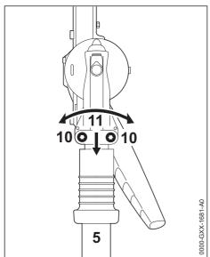
► Loosen the clamp screws (10).
